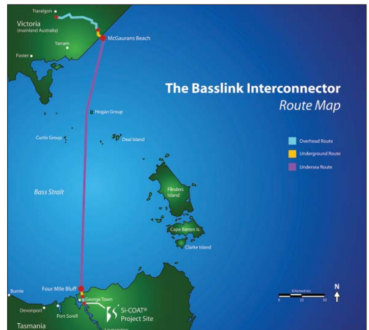
Si-COAT HVIC was applied to the DC side of the Basslink Interconnector Converter Station near George Town. ±400 kV DC electricity from the Converter Station is transmitted via overhead, underground and undersea lines to mainland Australia.
